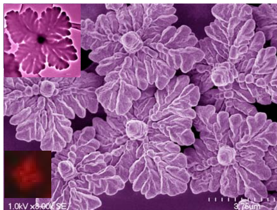
Figure 27. SEM image of porphyrin 'clover' formed by ionic self-assembly of two oppositely charged porphyrins. Upper Inset: TEM image. Lower Inset: Confocal image, showing preferential fluorescence from spines of the clover leaves.
