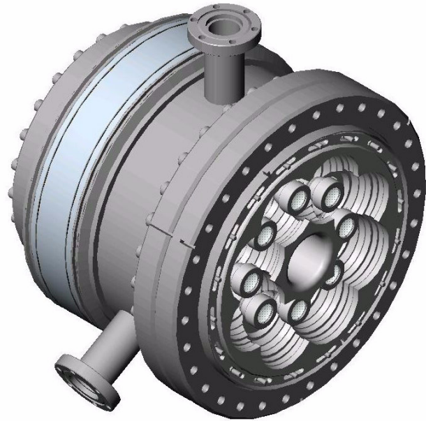
Figure 2. Configuration of the multiple beam electron gun currently under construction
