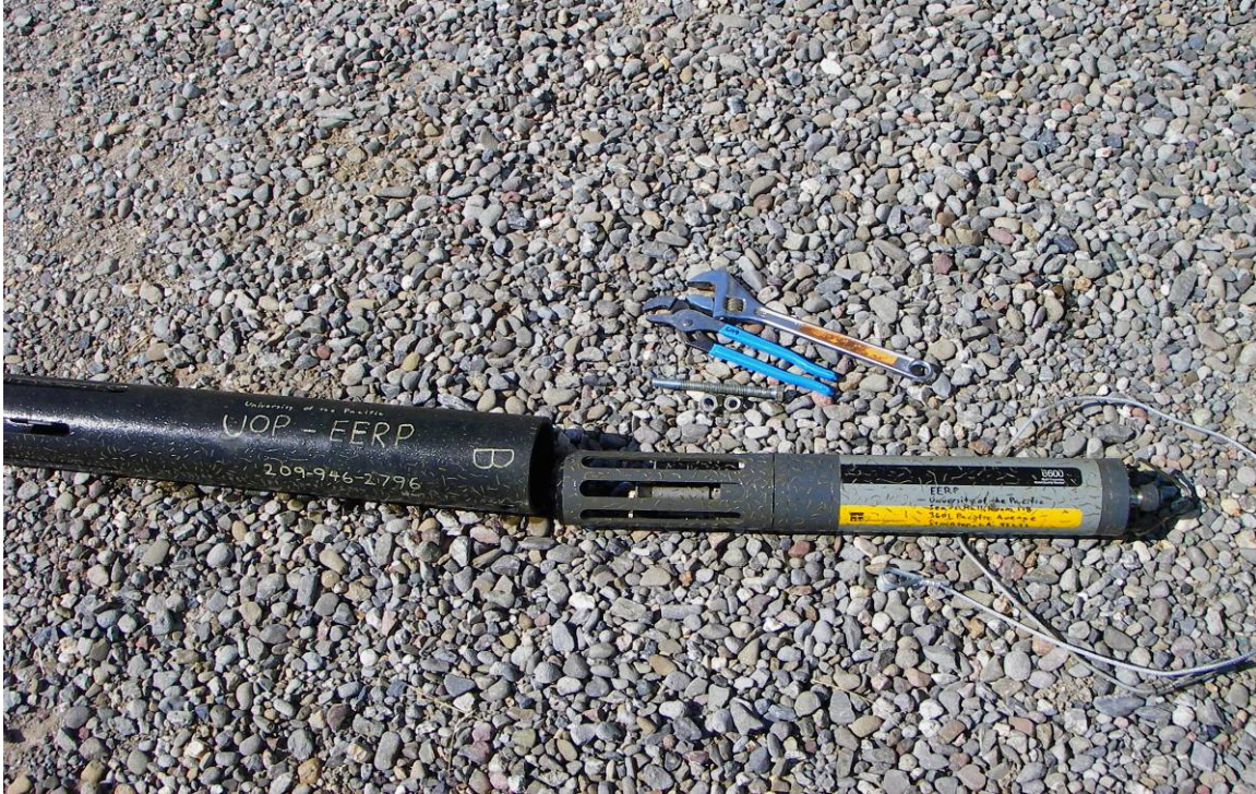
Fig.1 Waterquality Sonde with custom protective housing.
