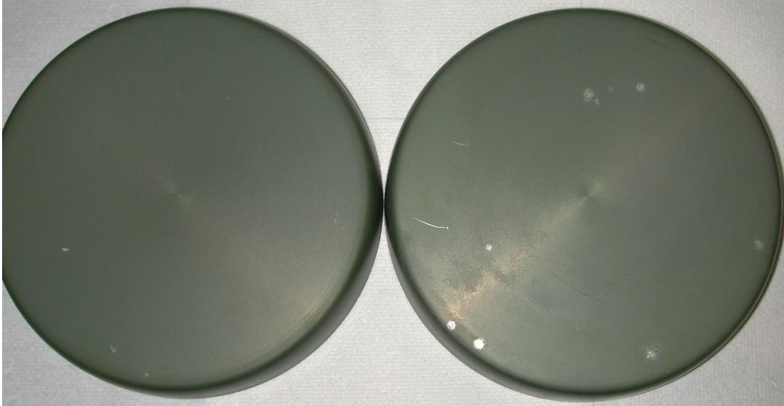
Figure 92. Photographs of chromium oxide coated 316L electrodes 1 and 2 after shot 96b of the 3 rd shots series labeled with blue diamonds in Fig. 85.
