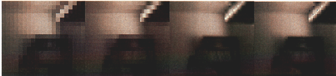
Figure 40: JPEG Compression. a) Image using only the first coefficient of the DCT matrix. Shows the mean value for each 8x8 pixel block. b) Image using the first two coefficients of the DCT matrix. c) Image using the first three coefficients of the DCT matrix. d) Image using the first four coefficients of the DCT matrix.
