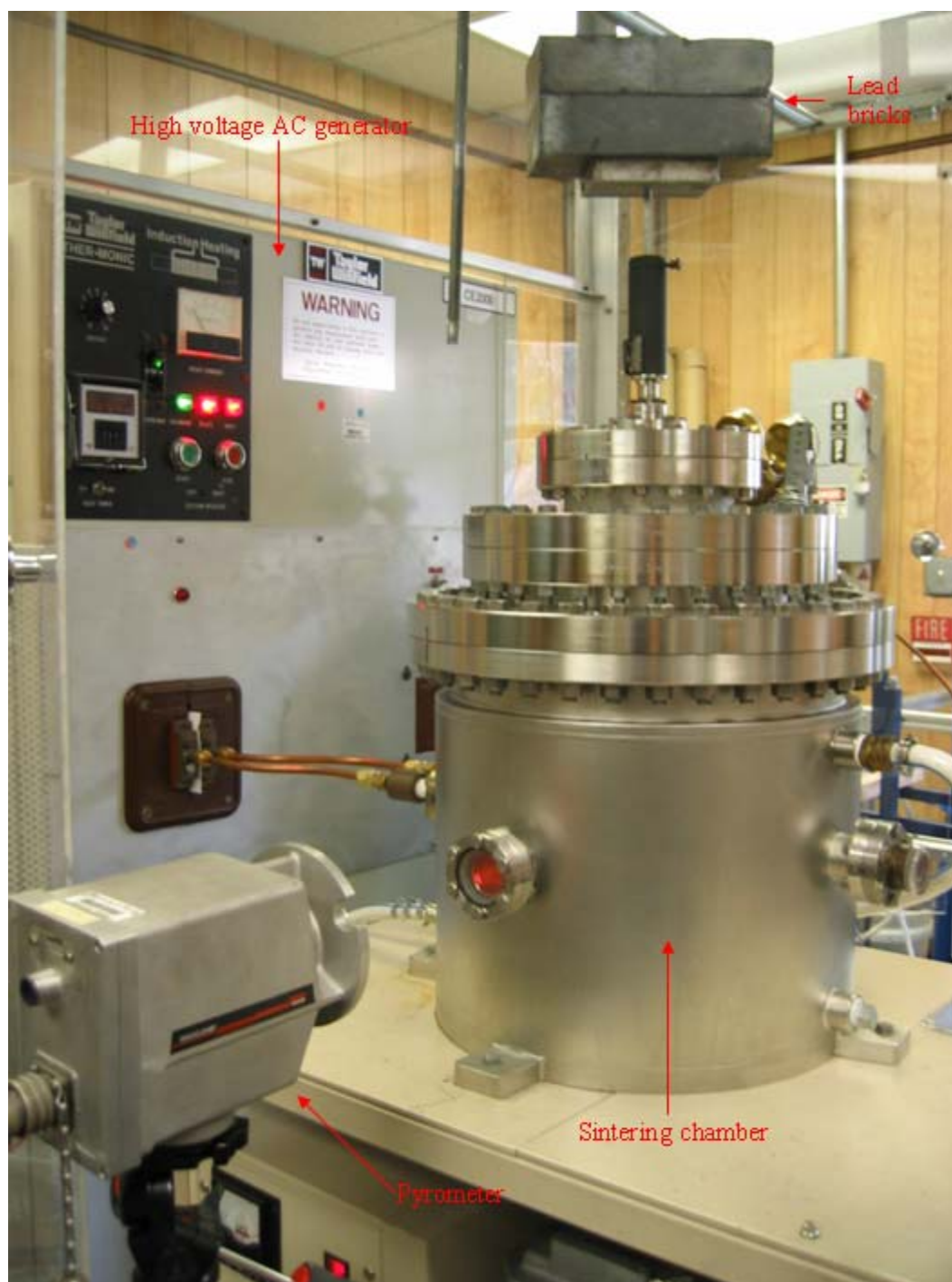
Figure 3-27. Hot Press Sintering Apparatus.
