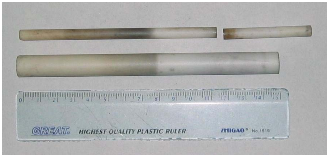
Figure 3-24. Alumina Die for Hot Press Sintering.
