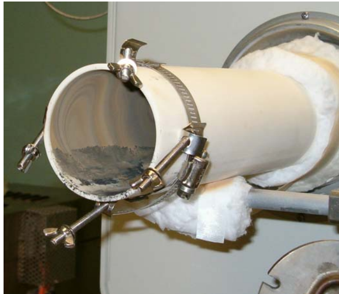
Figure 3-67. Furnace Tube after Carbonization and CVD process.
