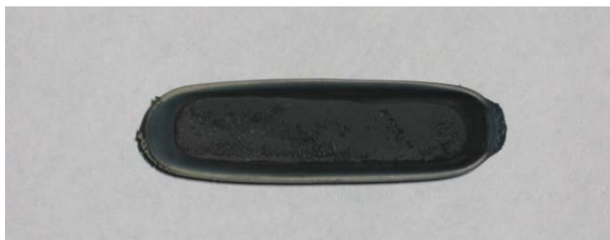
Figure 3-64. Uranium Dioxide Powder after CVD of SiC
