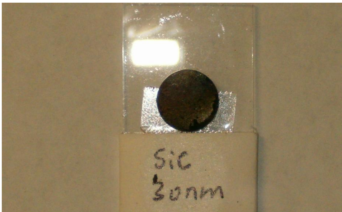
Figure 3-19. UO 2 -SiC pellet after sintering at 1300 °C
