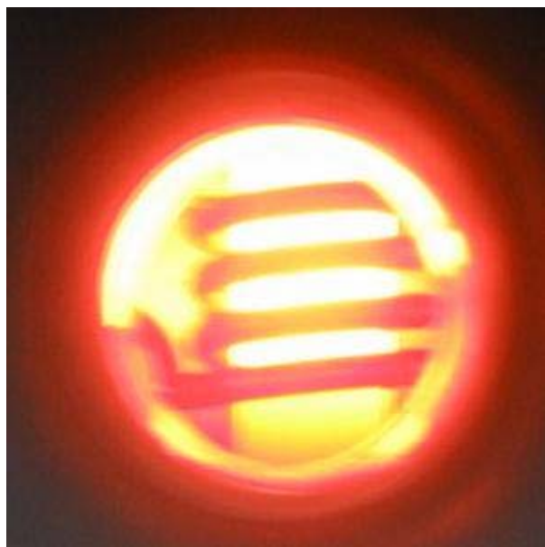
Figure 3-28. Heated Graphite Tube Observed Through the Pyrometer.
