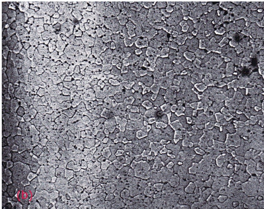
Figure 2-9. Microstructure of the Sintered \text{UO}_2 Pellets. (a), \text{UO}_2 Pellet Sintered at 1650^\circ\text{C} for 6 hours in \text{H}_2 . (X250) (b), \text{UO}_2 Pellet Sintered at 1300^\circ\text{C} for 1 hour \text{N}_2 , 1 hour in \text{H}_2 . (X250)
