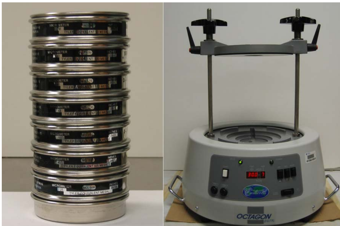
Figure 3-8. Sieve and Shaker for Analyzing Particle Size Distribution.
