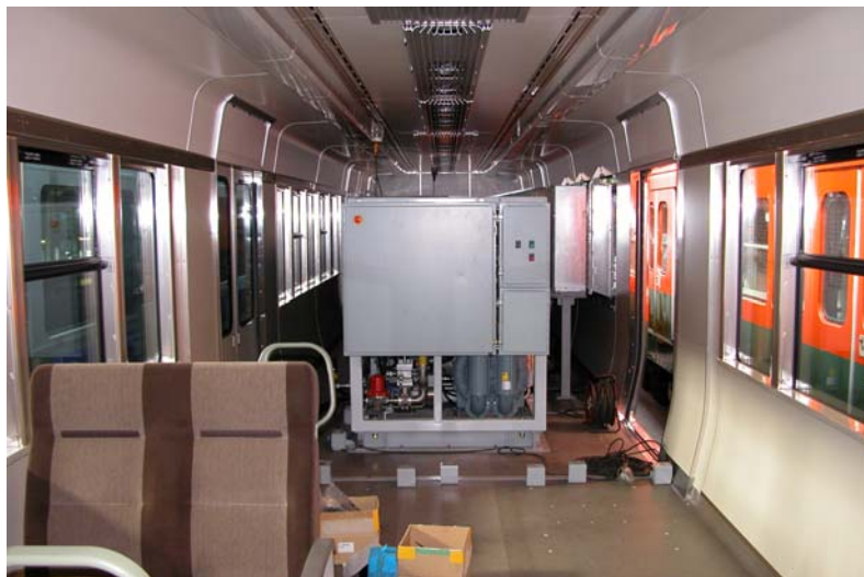
Fig. 3. 150 kW module installed in RTRI commuter train for testing.
