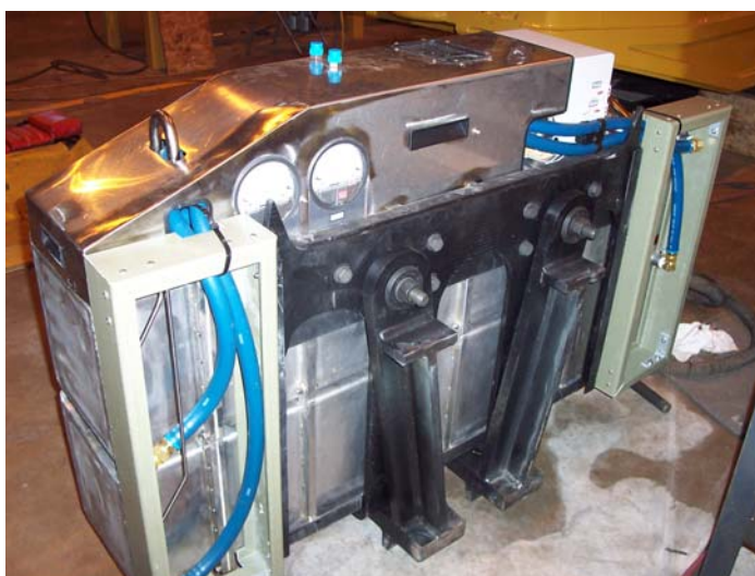
Fig. 4. One metal-hydride module with mounting guides.
