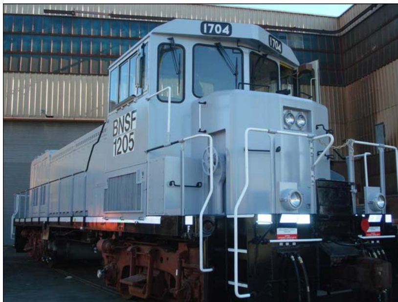
Fig. 8. BNSF battery-hybrid switcher locomotive platform.
