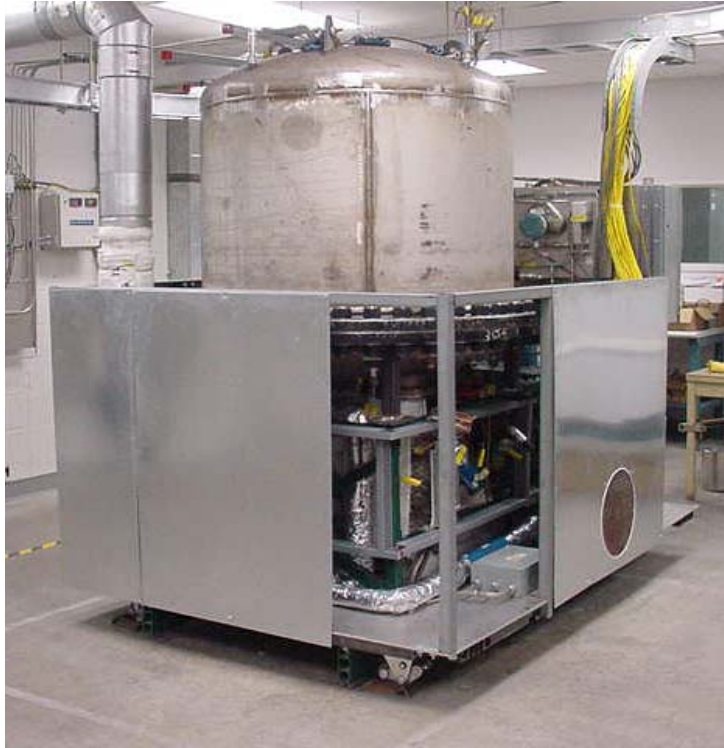
Figure 10.4. Completed prototype system for hot testing without SOFC stacks (one side panel removed for illustration).
