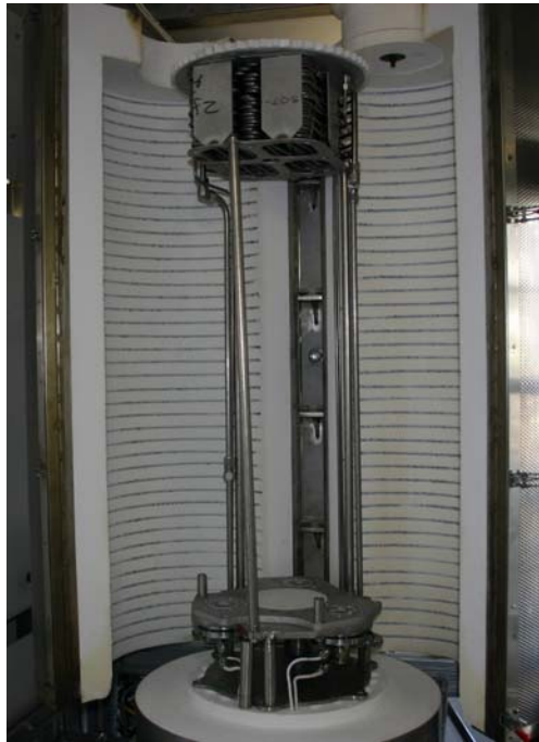
Figure 5.5. The fixture for building SECA system stacks. Here, it is installed into a test stand furnace.
