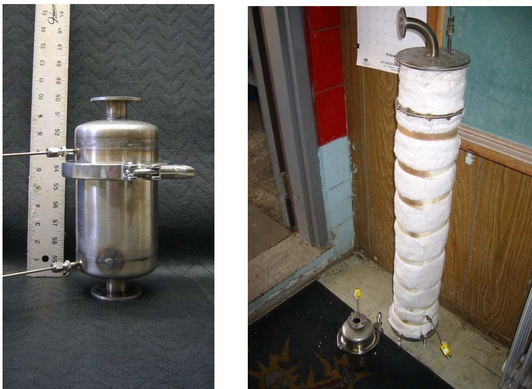
Figure 6.28 Photographs of the Fuel Processor Hardware. The photo on the left shows the redesigned fuel processor while the photo on the right shows both the old and new processors together.
