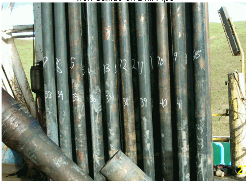
Iron Sulfide on Drill Pipe
