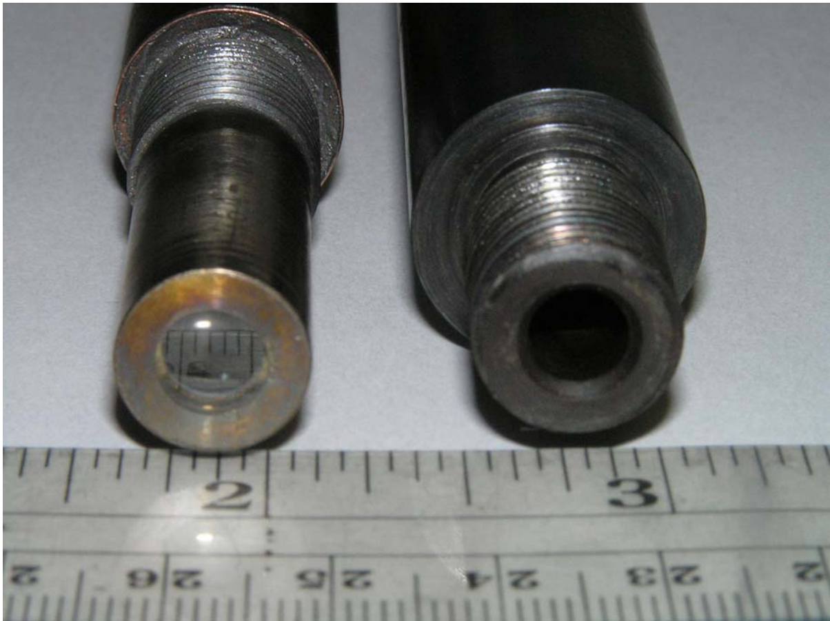
Figure 4.20: View of engine side of the sapphire window/lens (left) and the spark plug adaptor showing the optical access cavity (right)
