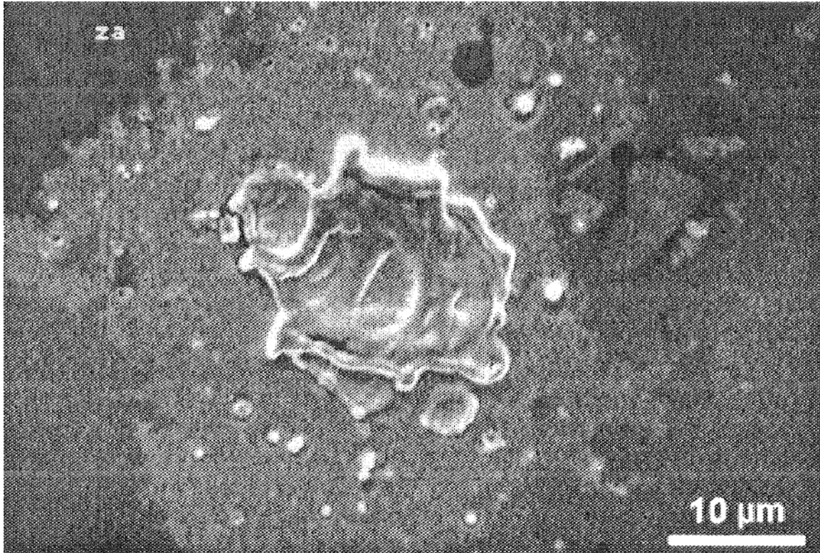
Figure 3.3: Cratering produced by a discharge across a 1 mm gap at 9 bars in air with a Platinum cathode [25]
