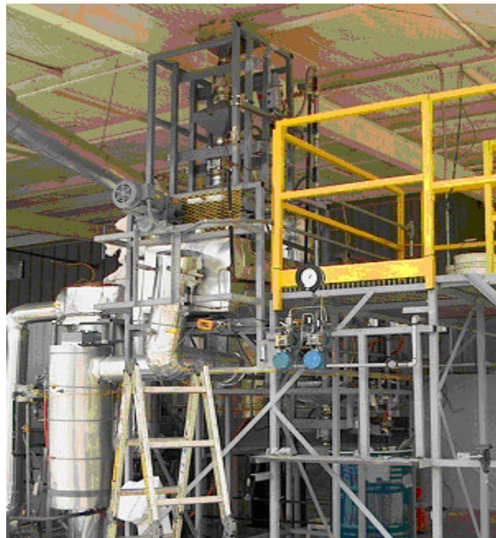
Figure 4 Pyrolysis Unit with Biomass feedstack system
