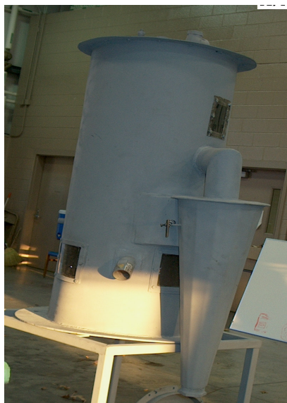
Figure 10 Photo of the char-fertilizer reactor
