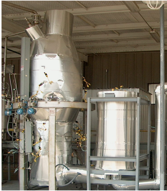
Figure 5 Fluidized Reformer and Pre-heater Unit
