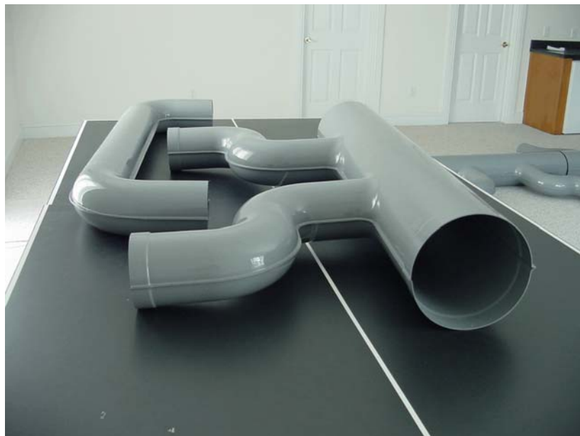
Figure 36 Duct halves made whole parts by bonding
