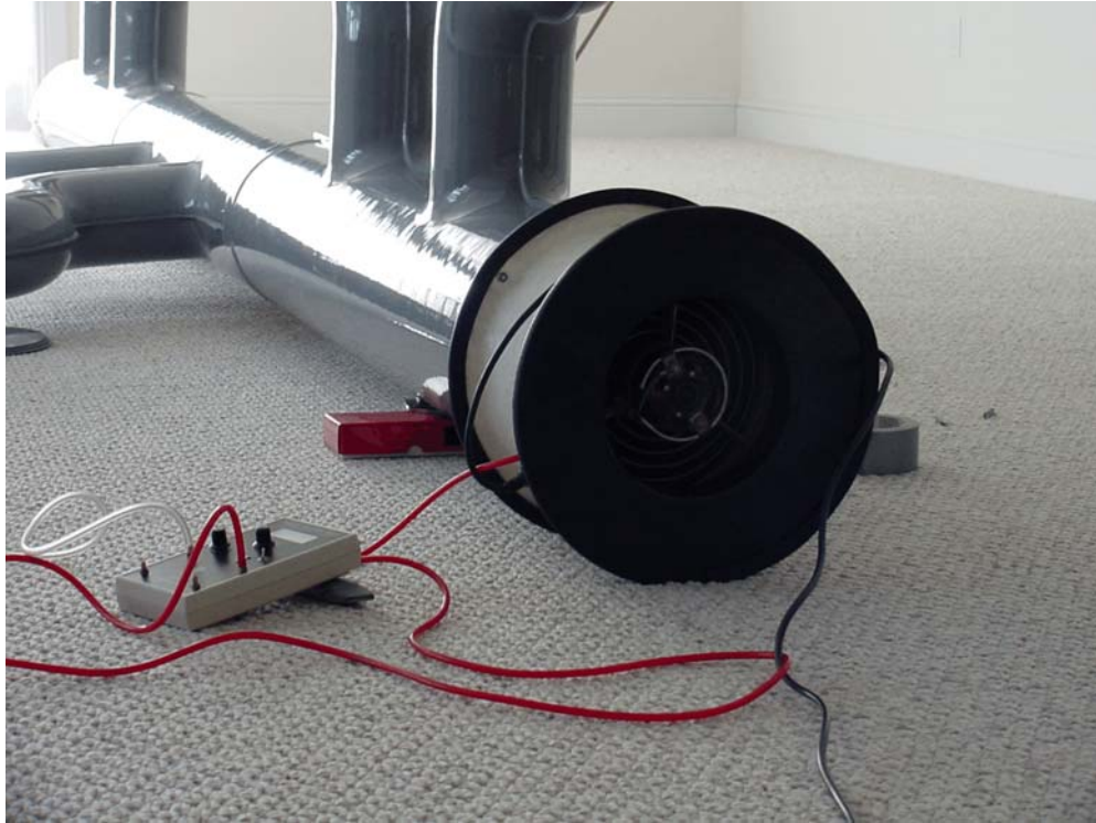
Figure 39 Duct Blaster hooked up to main trunk to measure air leakage
