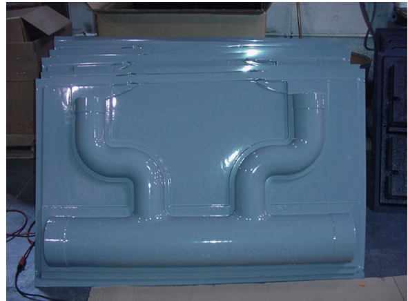
Figure 2 Thermoformed ductwork component, produced by SWA during Phase I research.
