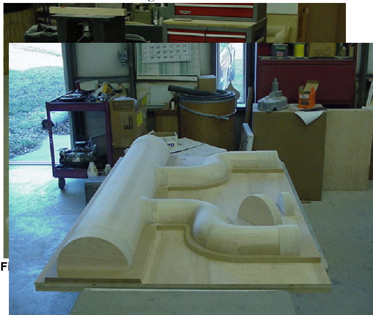
Figure 28 Wooden mold of half the main trunk
