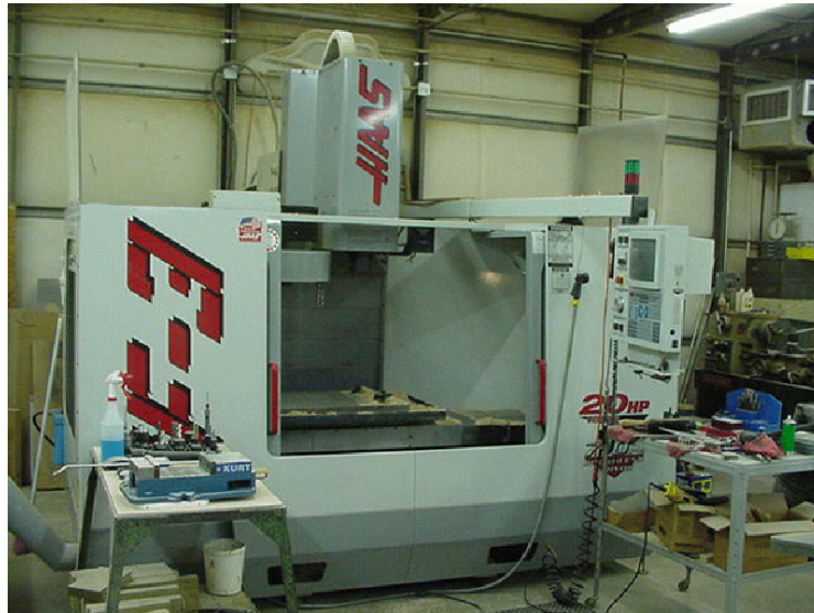
Figure 27 A vertical CNC milling machine used to machine prototype molds in Phase I
