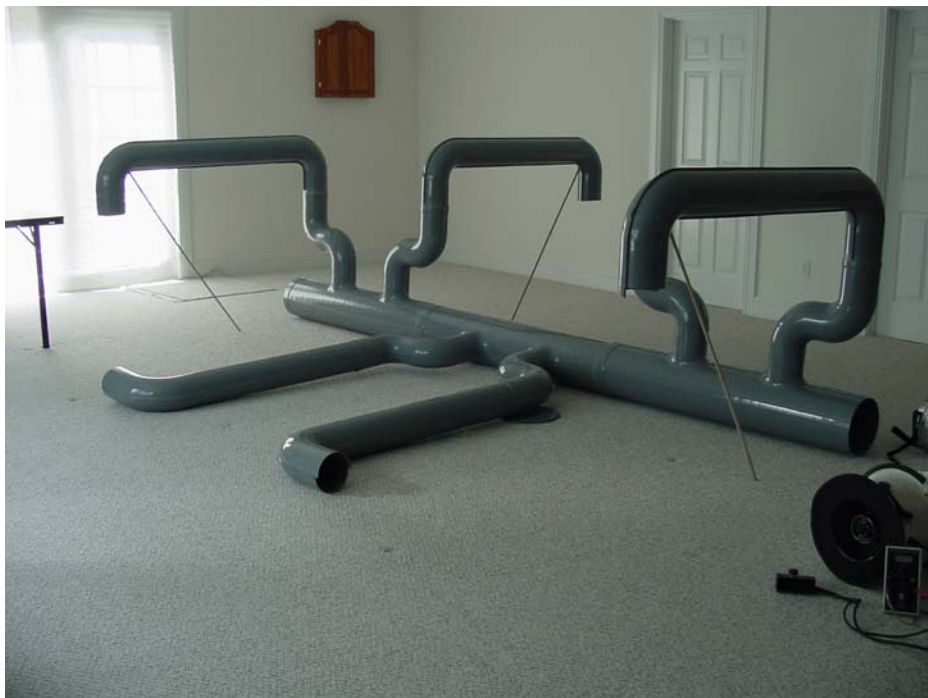
Figure 3 Assembled Phase I prototype duct system, all produced in two thermoforming molds. The system was virtually airtight.
