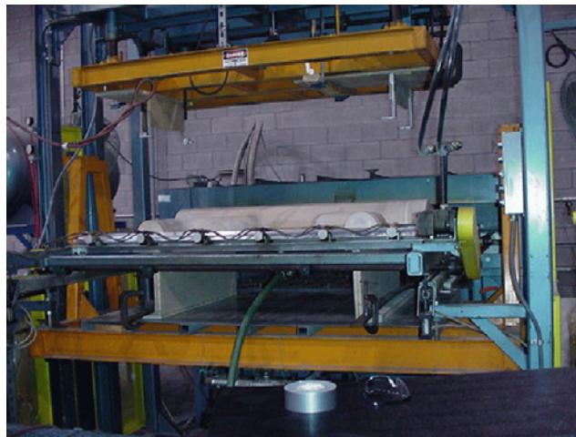
Figure 30 Single sheet thermoformer used to form the Phase I prototype duct components
