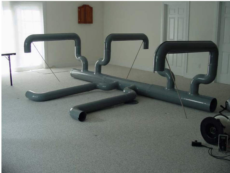
Figure 38 Assembled Phase I prototype duct system, all produced in two thermoforming molds. The system was virtually leakproof.
