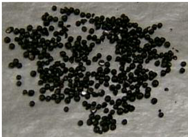
Figure 1. \text{Cu}/\text{Fe}/\text{Al}_2\text{O}_3 granular particles of \sim 1 mm in diameter.
