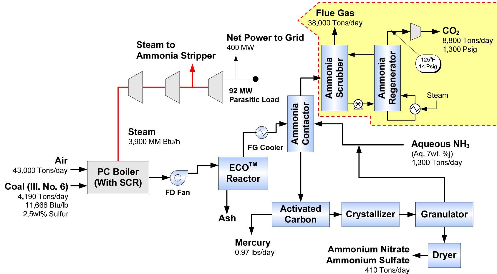
Integrated with Powerspan's multi-pollutant control ECO™ technology
