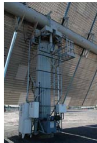
Figure 6-4. The 320-m 2 PV trackers at APS use hydraulic drives.
