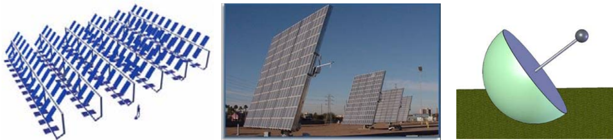
Figure S-5. In the mega-ganged heliostat proposed by DLR (left), up to ~500 m 2 of multiple facets are coupled via a common drive. In the mega-helio proposed by Arizona Public Service (center), an existing 320-m 2 PV tracker would be converted to a heliostat. The water-ballasted heliostat proposed by New Mexico Tech (right) is moved by pumping water between internal chambers. The ball at the end the post is a counterweight.
