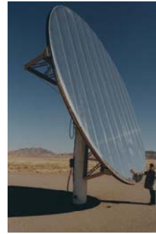
Figure S-3. Mid-1980s path to low-cost heliostats. Also shown are the 148-m 2 glass/metal (top) and 50-m 2 SM prototypes.
