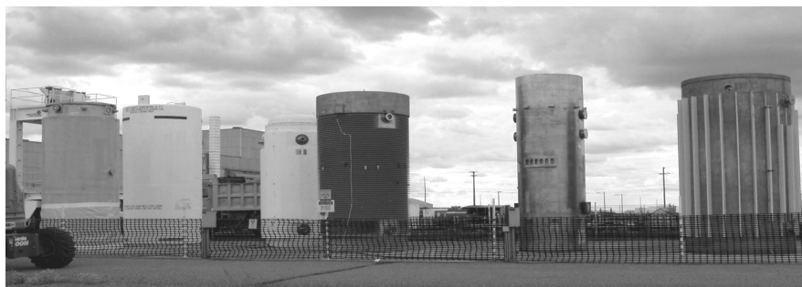
Figure 2. Commercial Dry Storage casks used in SNF tests at the INL Left to Right: REA 2023; VSC-17; TN 24P; V21; 125B; MC-10
