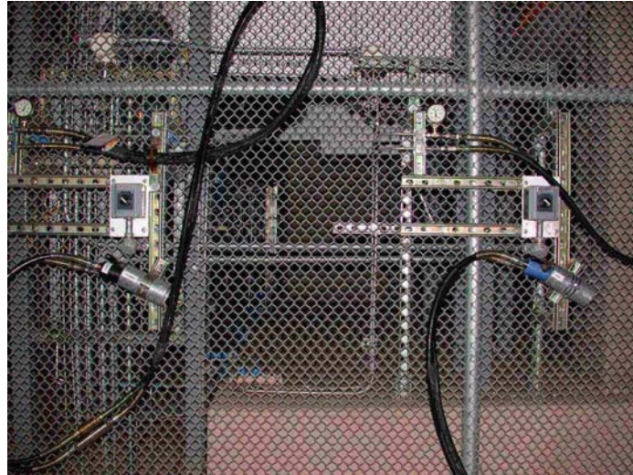
Figure 11. The 100% CNG and H/CNG nozzle is on the left; the 100% hydrogen nozzle is on the right. The nozzles are being used to fuel vehicles to test the prototype dispenser operations.
