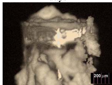
Figure 47. Images showing the range of film properties and adhesion obtained by varying the sol-gel aging time and co-solvent. The binder composition is 55% OtMOS / TEOS and the diameter of the particles are 1-8 \mu\text{m} for all samples shown.
