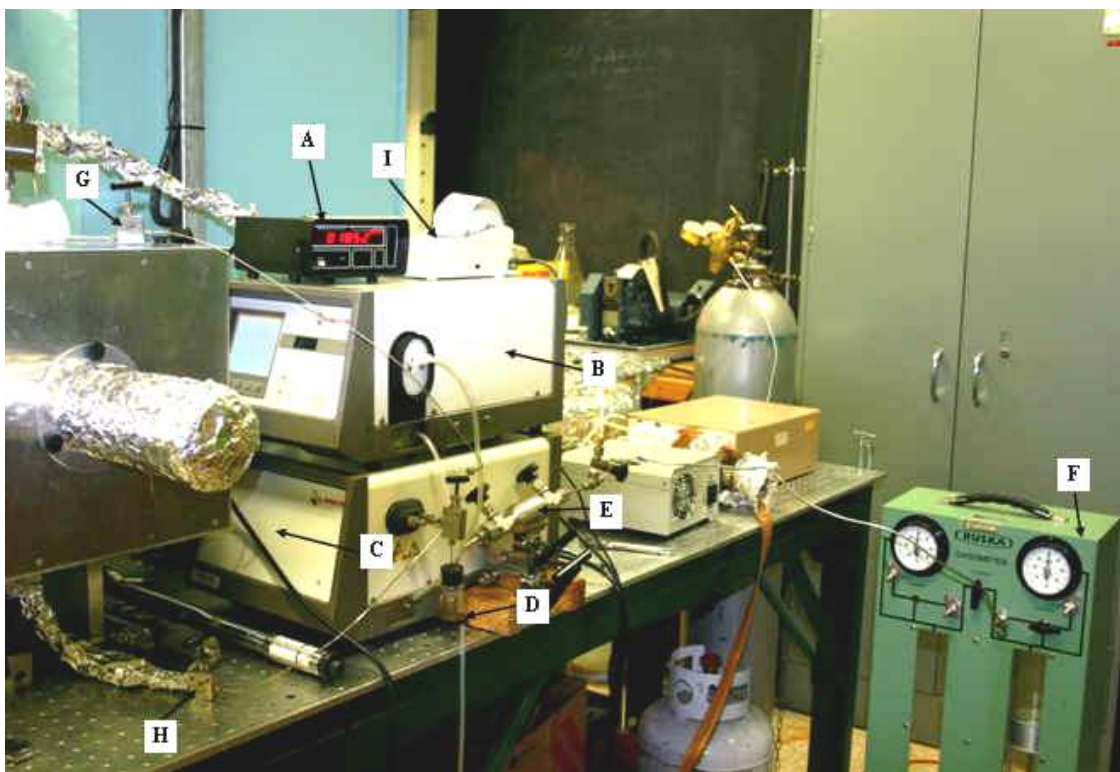
Figure 2.19: Pressure densitometer and flash separation unit
