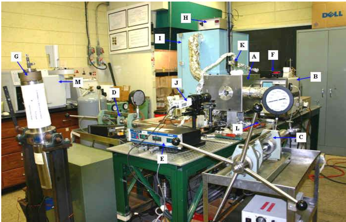
Figure 2.21: Various equipments used for measuring interfacial tension at different experimental pressures at 238°F
