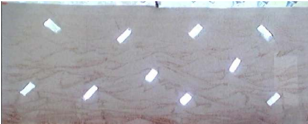
Figure 1.42: Oil-Wet Physical Model after Immiscible GAGD
