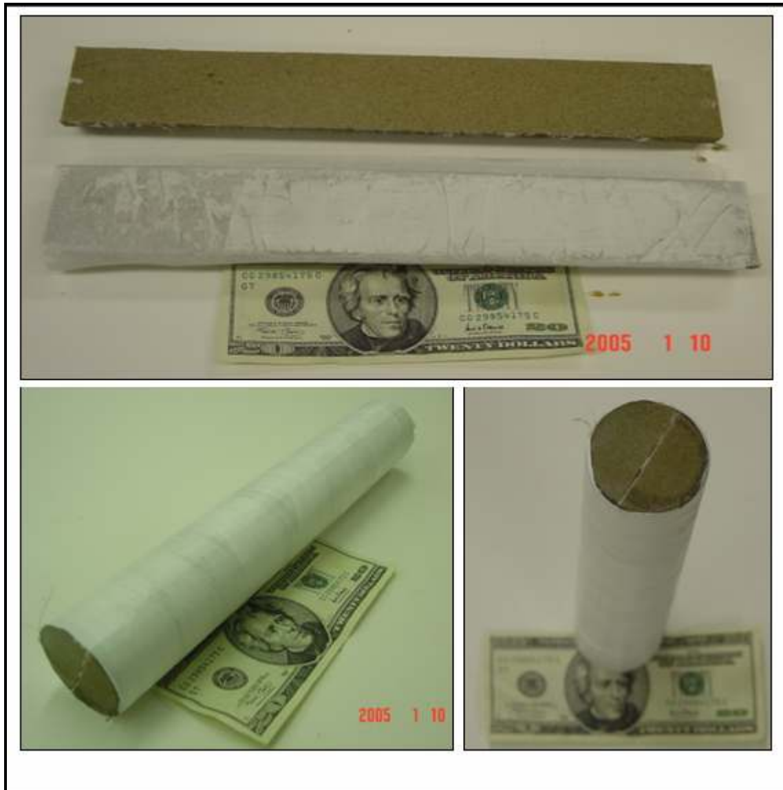
Figure 3.66: Pictures Showing Sliced Berea Core with Sand Pattie and Kim-wipes® for Capillary Contact (Top) and the final assembled core with a central 15-D perm fracture
