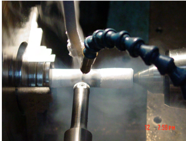
Figure 7.22. Experimental setup for ultrasonic surface modification at cryogenic temperature
