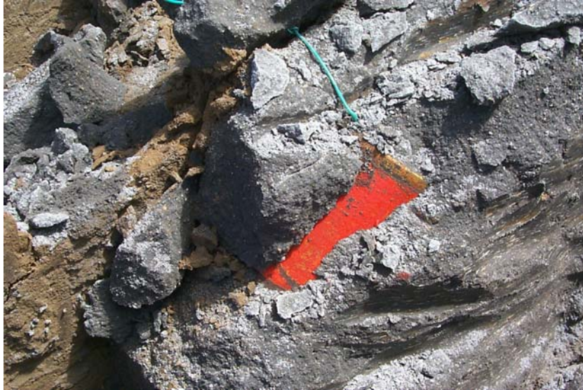
Figure 31. Photograph of Pipe Embed Being Excavated From Flowable Fill
