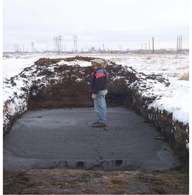
Figure 27. Short-Term Performance of 10E200-Grade Fill After 16 Hours
