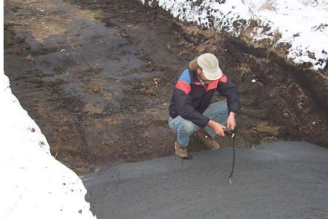
Figure 24. Monitoring of the Temperature of the 10E200 Flowable Fill After Placement
