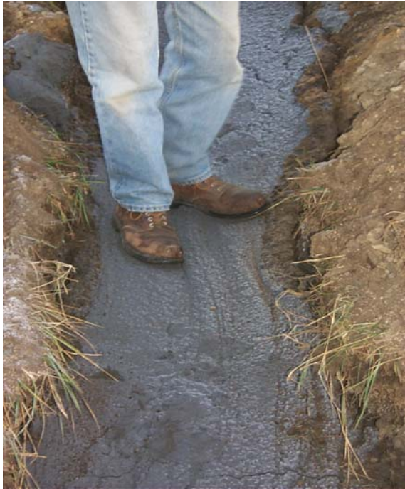
Figure 26. Ability of the 30E-Grade Fill to Support a Person After 16 Hours
