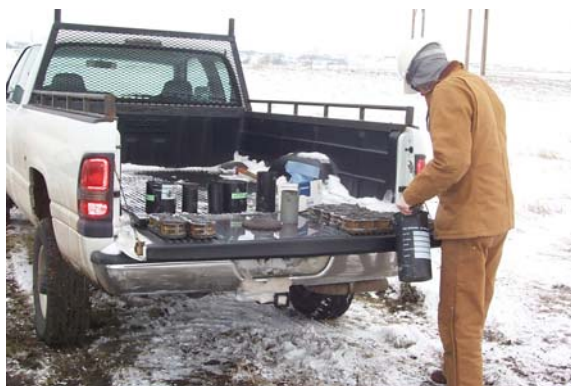
Figure 25. Collection and Fabrication of Test Specimens in the Field During the 10E200 Demonstration
