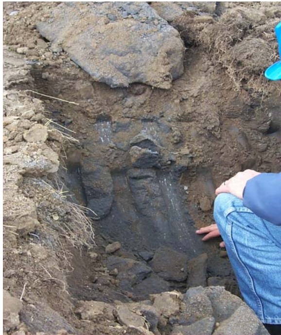
Figure 30. Photograph Showing the Cutting of the 30E Flowable Fill Material with a Toothed Bucket Backhoe
