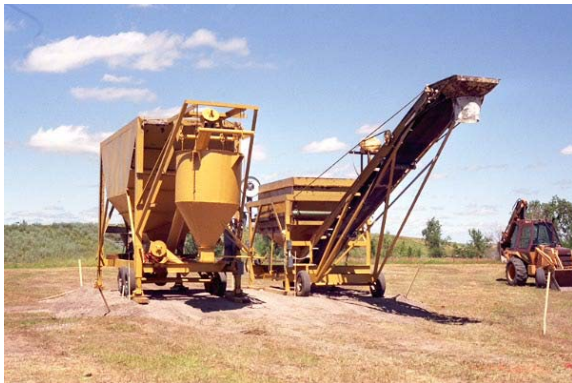
Figure 36. Placement of the Sand Hopper (Right) and Ash Hopper (Left)
