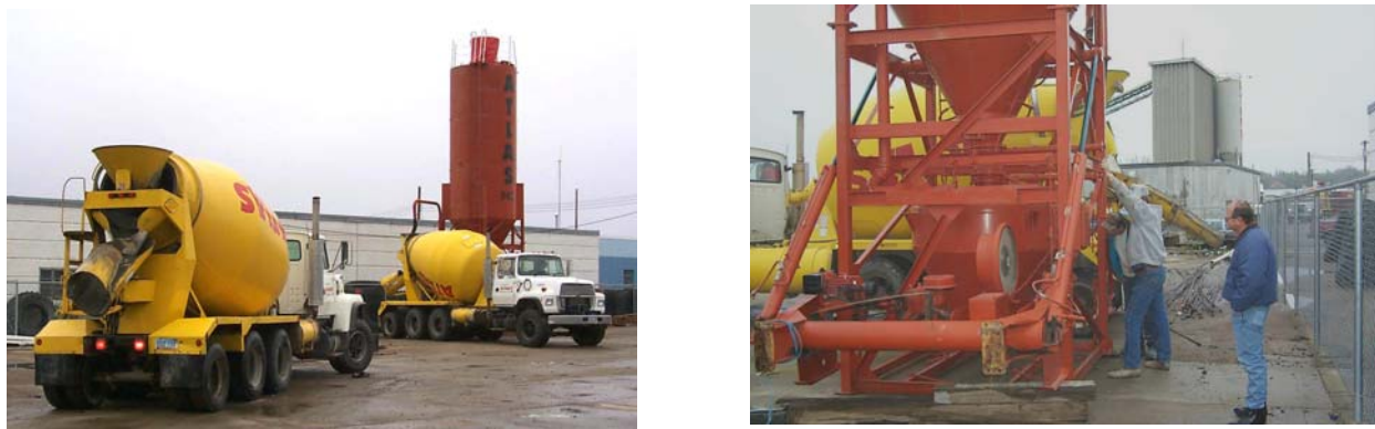
Figure 7. Photographs of the MDU Fly Ash Silo and Weigh System Erected at Atlas Ready-Mix for the Demonstrations
