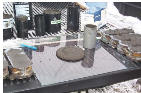
Figure 25. Collection and Fabrication of Test Specimens in the Field During the 10E200 Demonstration
