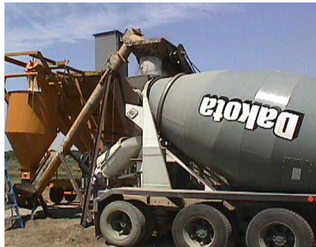
Figure 39. Photographs of the Batching and Loadout of the Ready-Fill Product
