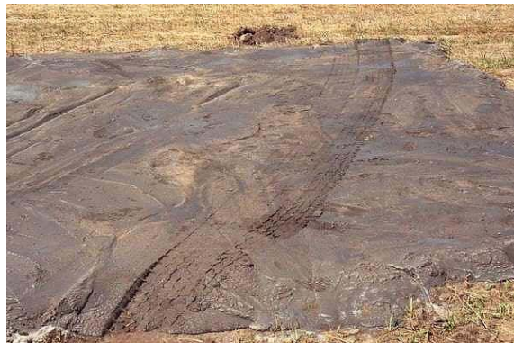
Figure 41. Pick-Up Truck Tire Track Indentation on Excavatable-Grade Ready-Fill After 24 Hours
