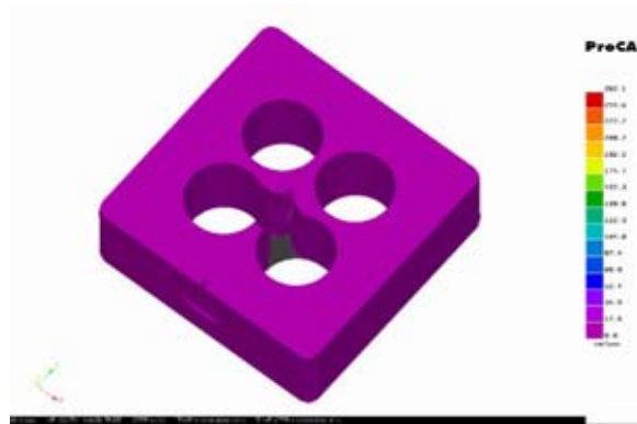
Figure 40. ProCAST prediction of the completed fill using a trapped-gas model.
