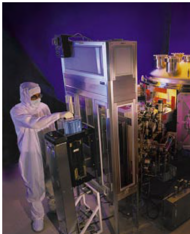
Ultra Clean Ion-Beam Sputter Deposition System that will be used in EUVL development to deposit thin films in integrated circuits
