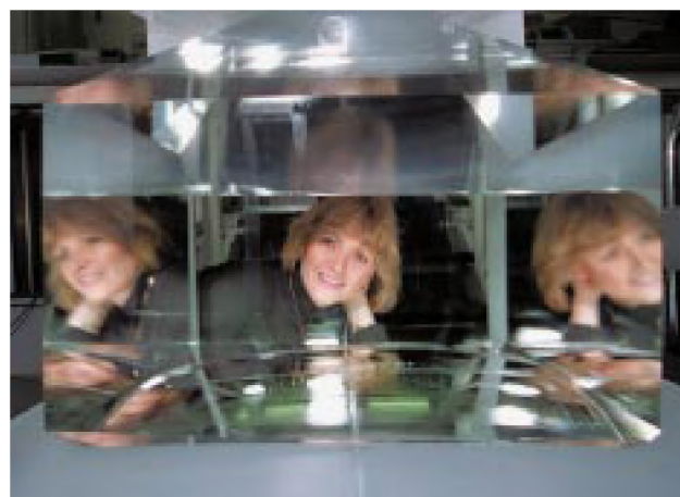
Potassium dihydrogen phosphate (KDP) crystal created with rapid-growth method.
