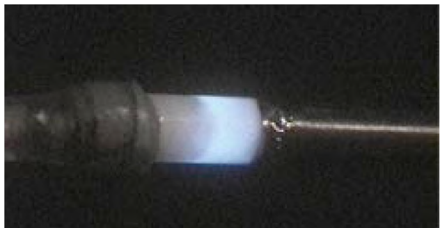
LLNL's x-ray catheter prototype, emitting a therapeutic x-ray dose ( >6\text{ Gy/minute} ).
