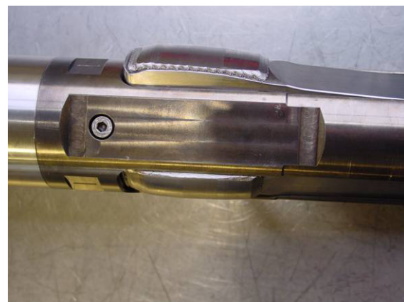
Figure 6: RSM ribs retracted (upper) and extended by 8mm (lower).
