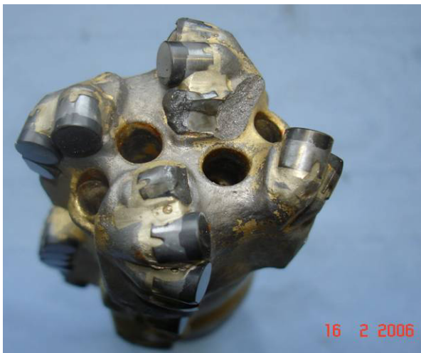
Figure 11: Damaged bi-center bit (broken blade)
