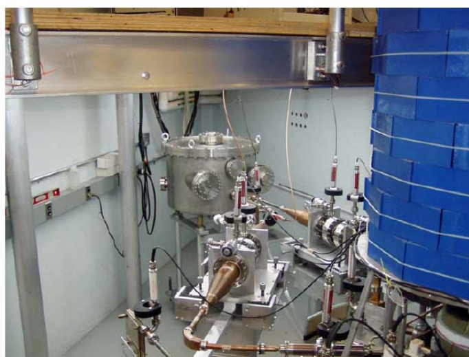
Fig. 1. Photographs of Omega-P 34-GHz magnicon, with windows and transmission lines.
