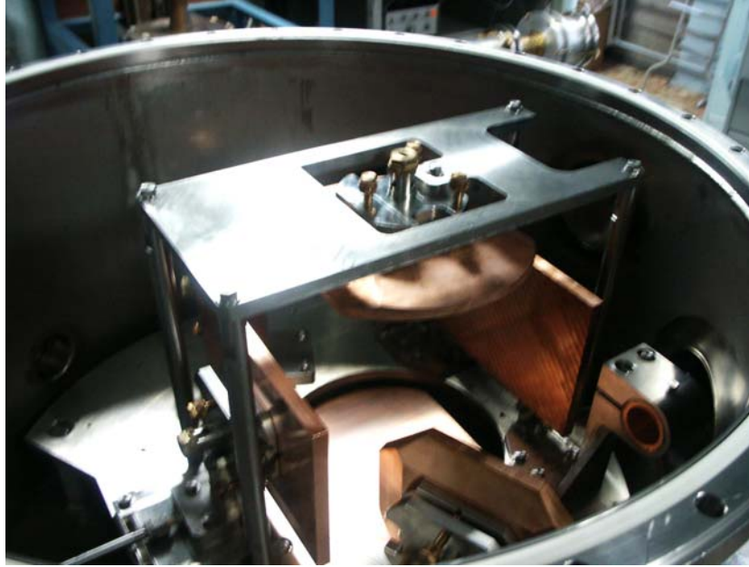
Fig. 31. Disposition of the mirrors of the four-mirror resonator in the vacuum chamber.
