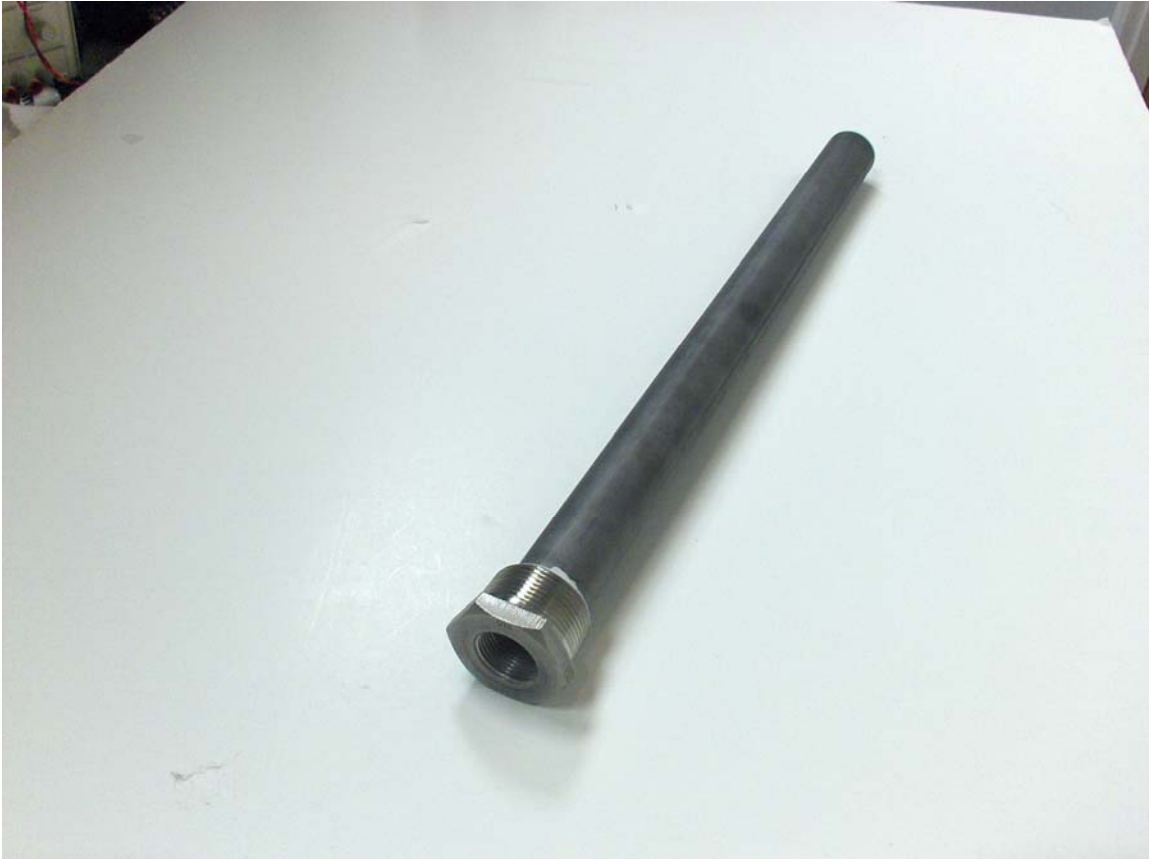
Fig.12 Example High Pressure High Temperature Seal SiC Tube that forms the basis of the SiC chip front-end packaging.
