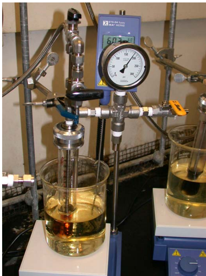
Figure D1: Low pressure (60-180 psi) ethenolysis reactor
