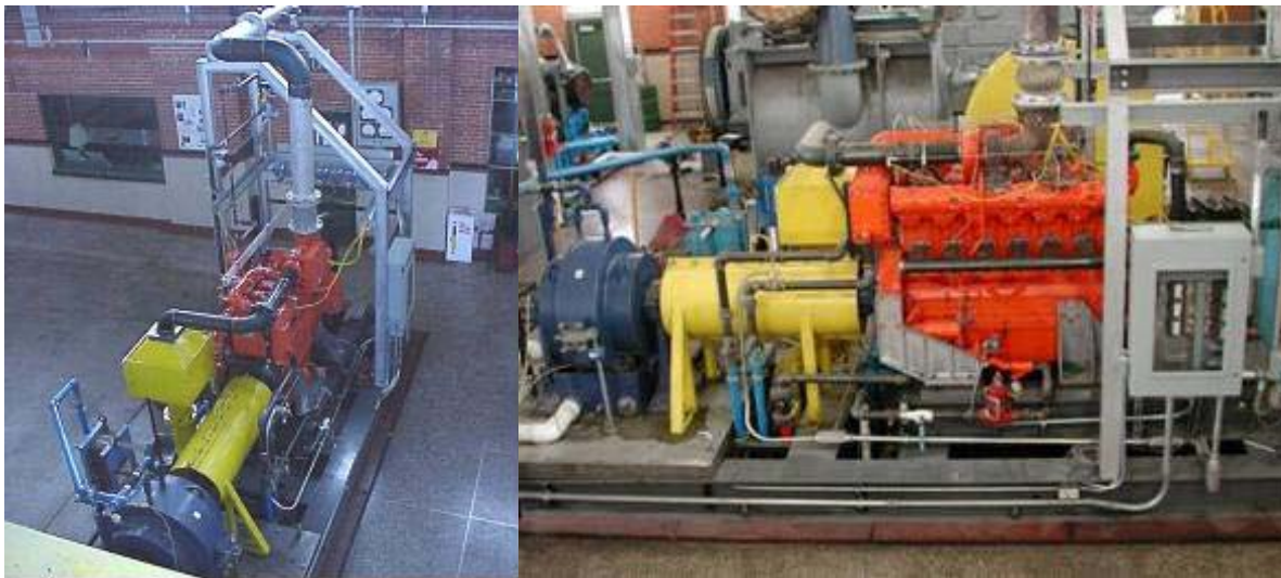
Figure 13-1: Waukesha VGF-F18G Installed at the Large Bore Engine Test Bed at Colorado State University
