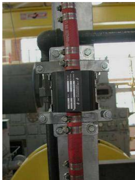
Figure 13-7: J-Tec Associates VF563B In-Line Blow-by Meter
