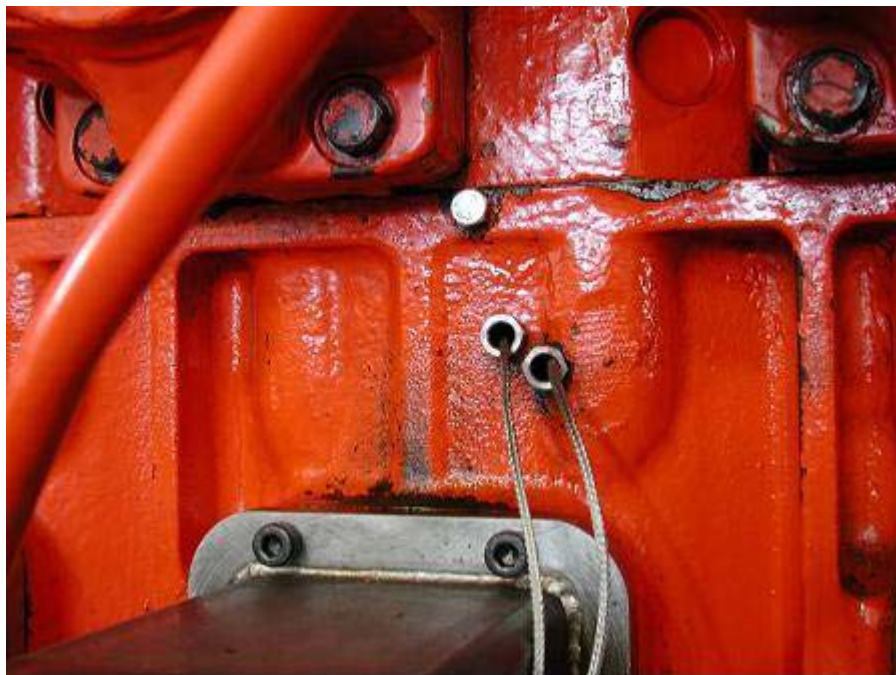
Figure 13-8: Inter-ring Pressure Transducers Installed on Engine
