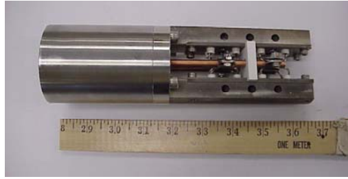
Figure 3-28 - The Getter Module Assembly for the Demonstrator
