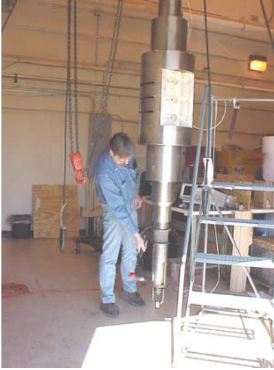
Figure 3-29 - Impact Modal Test on the Rotor Subassembly
