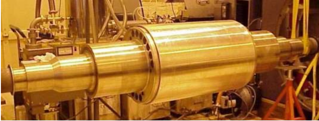
Figure 3-22 - The Demonstrator EM Shield Assembly
