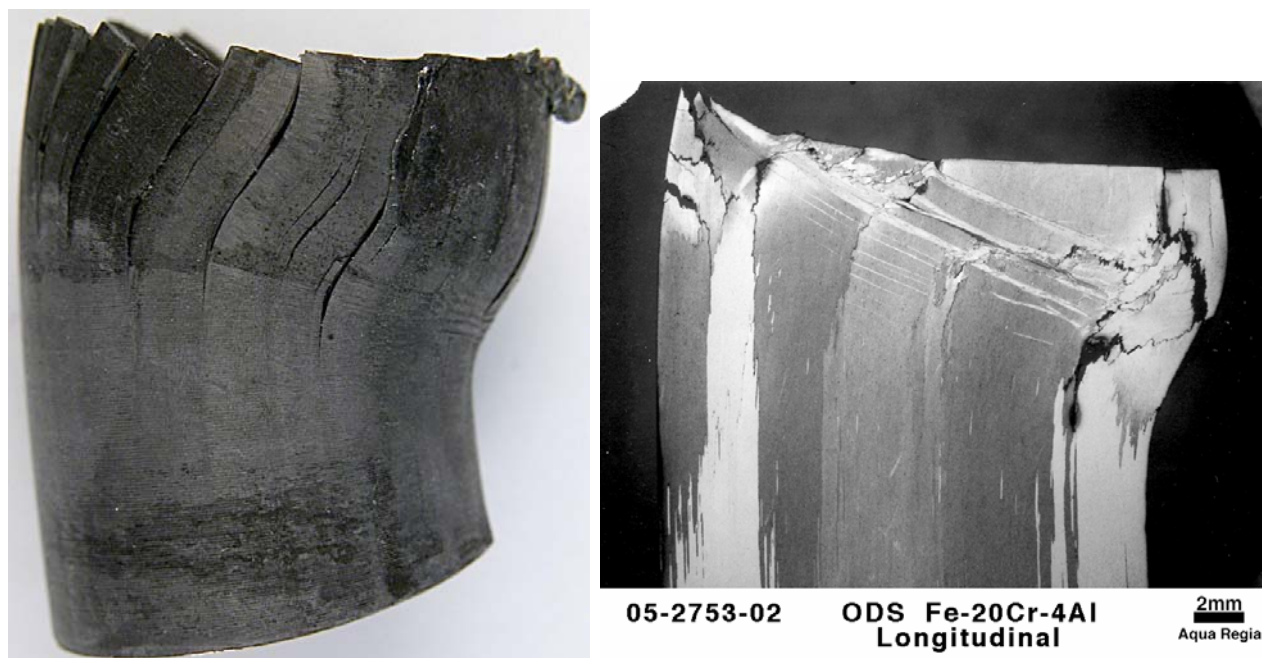
Figure 9: Macrostructure of Bonded Sample Overpressed during Joining
