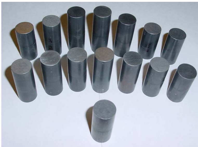
Figure 26: Bonded MA-956 and PM2000 Samples for Creep Testing at WMT&R
