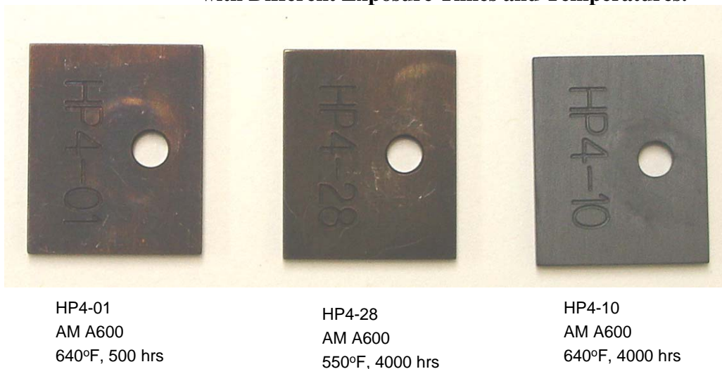
Figure 2: Comparison of Optical Heat Tints on As-Machined (AM) Alloy 600 Specimens with Different Exposure Times and Temperatures.
