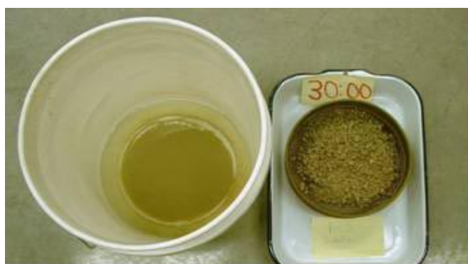
Figure 5: On the right is the Tyler 10 mesh screen holding the previously immersed agglomerates. The bucket on the left contains the fines which have been released due to the breakdown of the agglomerates.
