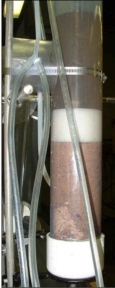
Figure 27: This photograph shows the ponding effects due to fines migration in scenario 3. A large amount of solution can be seen in the column above the ore and the overflow break over point (the Y fitting at the upper left corner).
