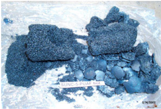
Figure 158 – Suncor Anti-Foaming Runs – Coke Picture (SUN 5 PUAF Bottom)
