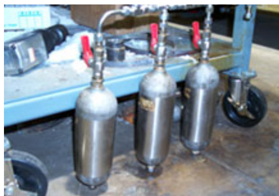
Figure 10 - Liquid collection system with Hoke cylinders and quick disconnect valves
