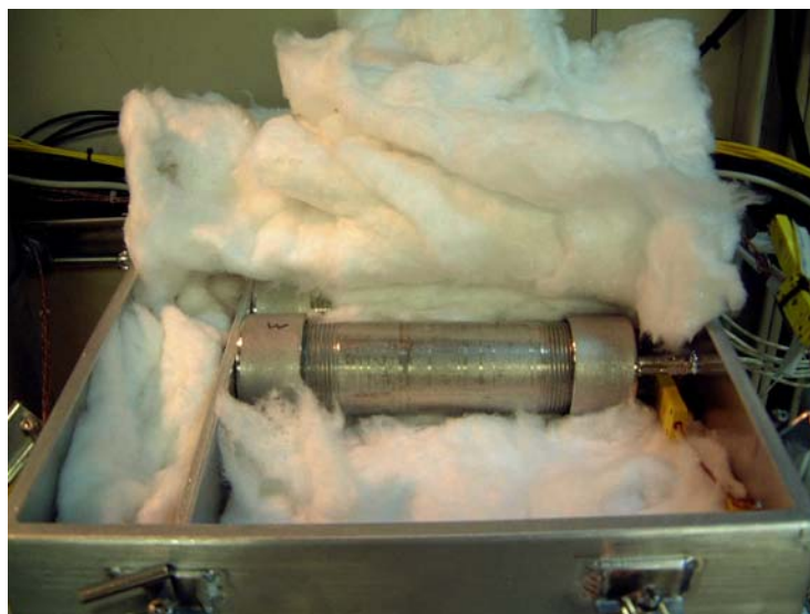
Figure 7. Heater assembly installed in insulated pipe nipple. Six of these are installed in the insulated box.
