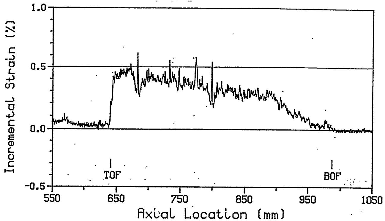
Fig. 1 Transient cladding strain for an element (P43-D79) from the 1C test. The element had high fuel smear density (91% TD), thin cladding (0.25 mm) and incurred no significant fuel melting. The cause for the strain was mainly fuel/cladding differential thermal expansion. TOF and BOF denotes top-of-fuel and bottom-of-fuel.
