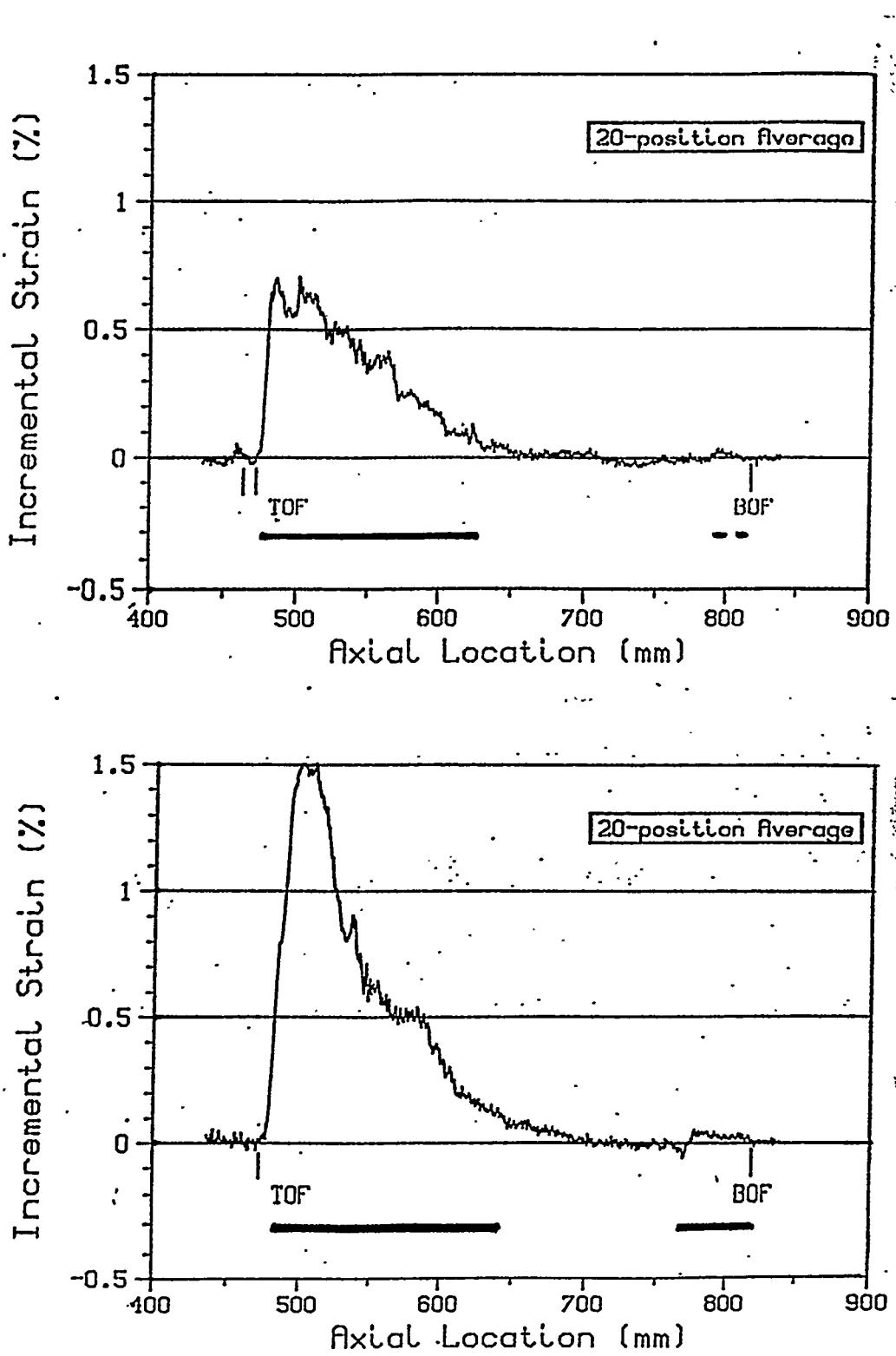
Fig. 4 Comparison of transient cladding strains between elements WT179 (top, with cavity pressure relief from molten fuel expulsion into the plenum) and WT180 (bottom, with no pressure relief). Both elements had PNC316 cladding and same aggressive design features. The horizontal bars denote the locations of the central cavities (determined from the posttransient radiographs).
