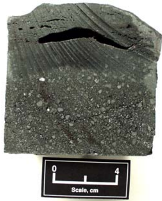
Fig. 6: Spalling in a refractory material
