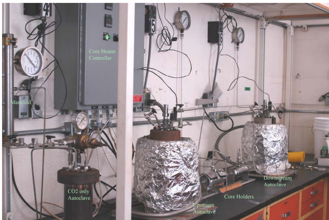
Figure 4. High pressure CO 2 flood test apparatus.
