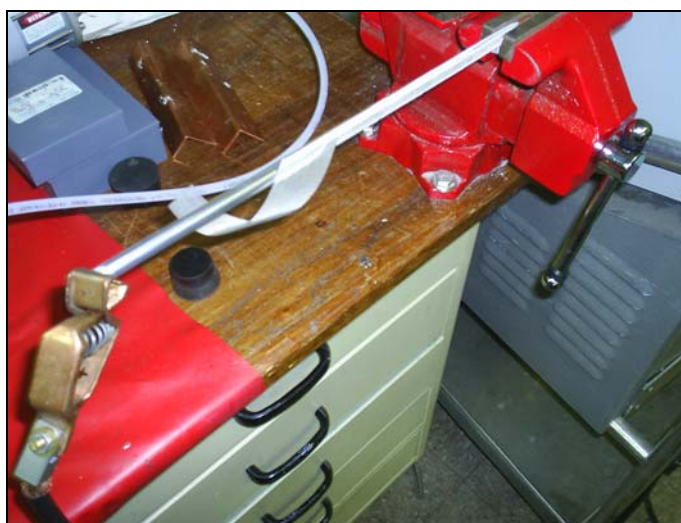
Figure 4.1. The bias wrapped wick.
