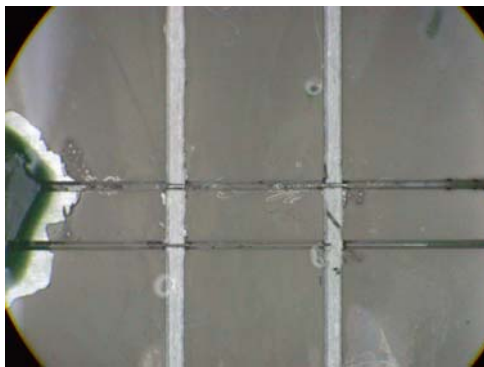
Figure 26. Inconel pad with fibers, after Nickel plating, ready for dicing.
