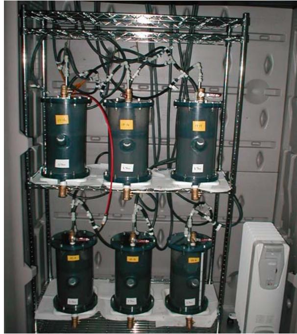
Figure 2.4. Six digesters housed in a temperature-controlled environment.
