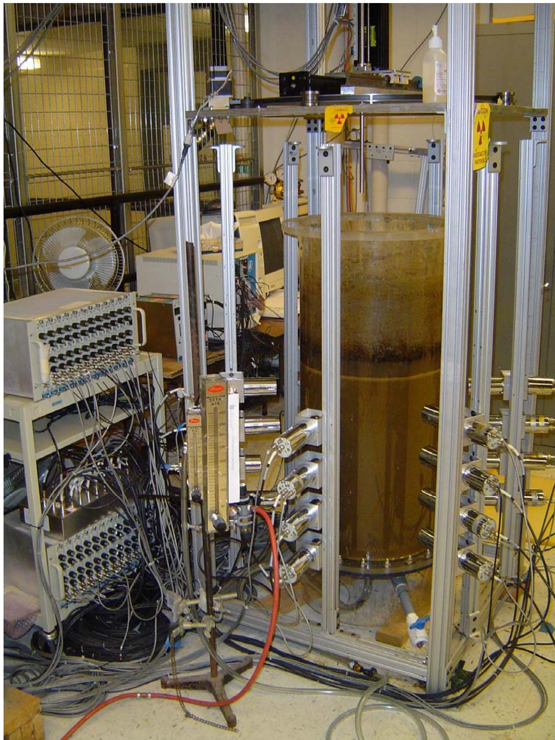
**Figure 4.4** Photograph of CARPT set-up for pilot-scale digester
