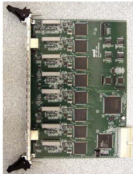
**Figure B.26** Pulse processor module.
