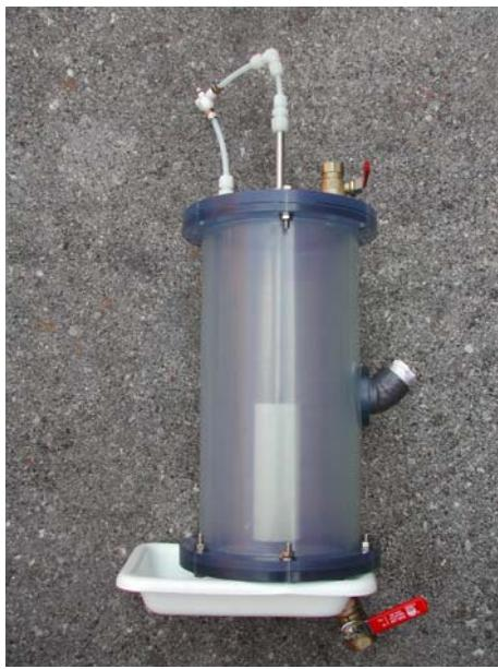
Figure 2.3. A Photograph of one of the anaerobic digesters used. From left to right the connections on top are gas outlet, gas inlet, and feed addition.
