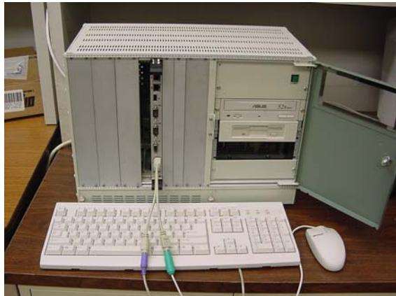
**Figure B.23** CPCI crate and single board computer.
