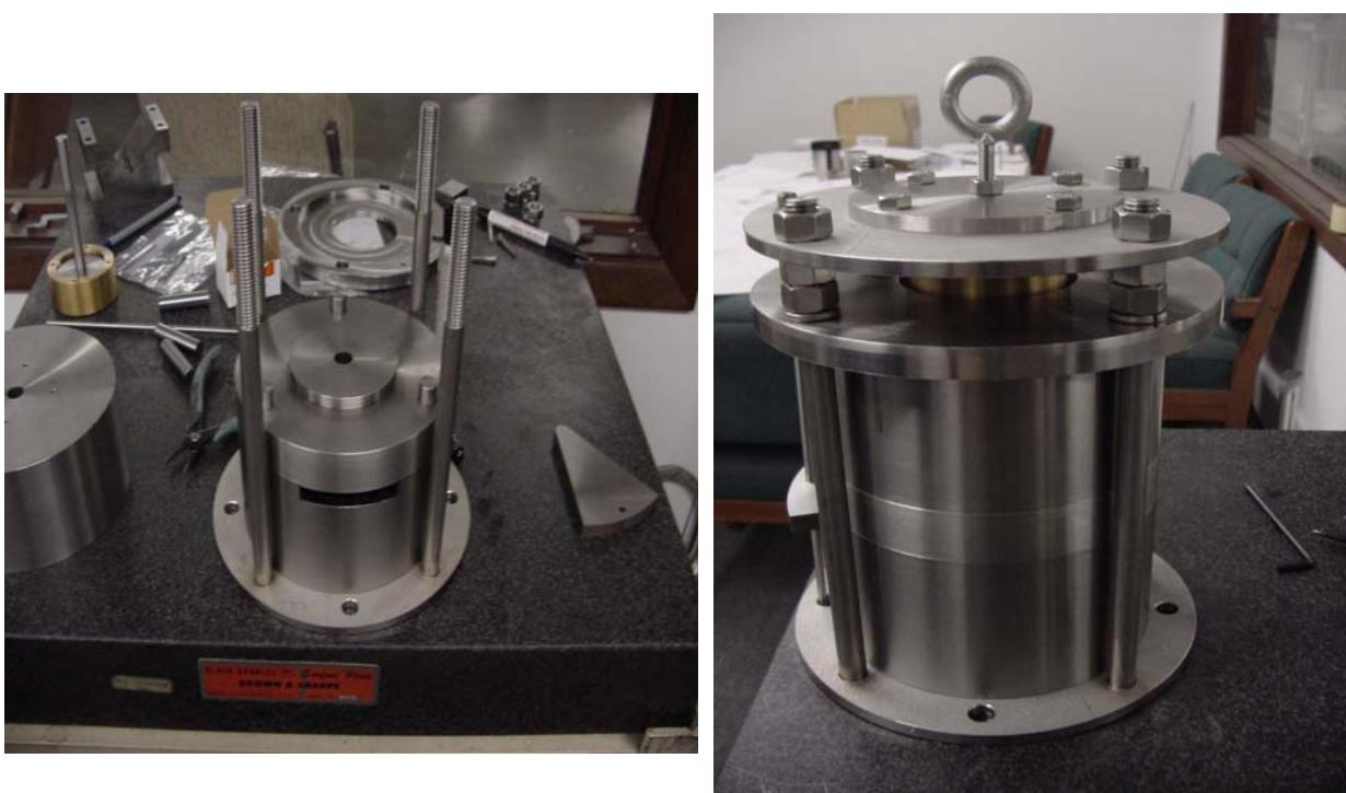
Figure 4.9: Tungsten collimator to house up to 100 mCi  $\text{Co}^{60}$  source
