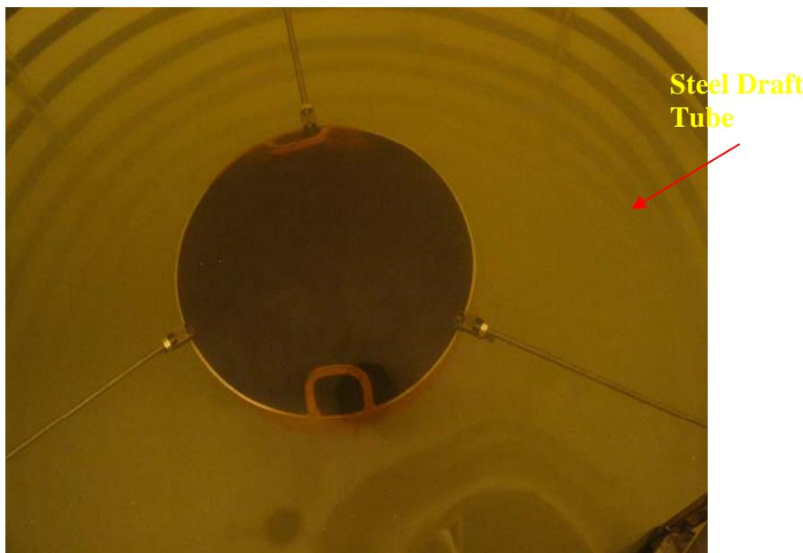
Figure 2.20: The top view of the reactor as seen through a man hole. The steel draft tube is visible in the center; it is supported by three tie rods.
