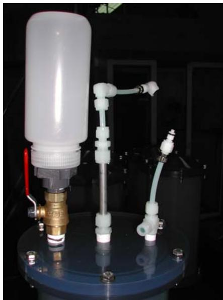
Figure 2.6. The slurry was fed through the top of the digester via a ball-valve.
