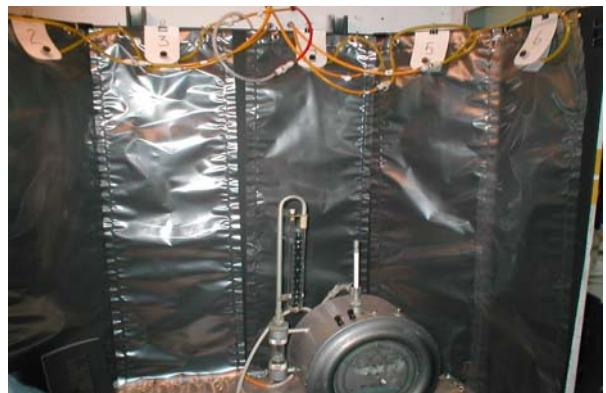
Figure 2.5. Gas bags for collecting biogas and wet gas test meter for measuring amount of gas generated.
