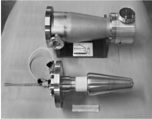
Figure 1: High voltage shielded, axial neutron generator shown with its target assembly separated from the main vacuum chamber. The short, 50 mm high voltage insulator is shown in the picture.
