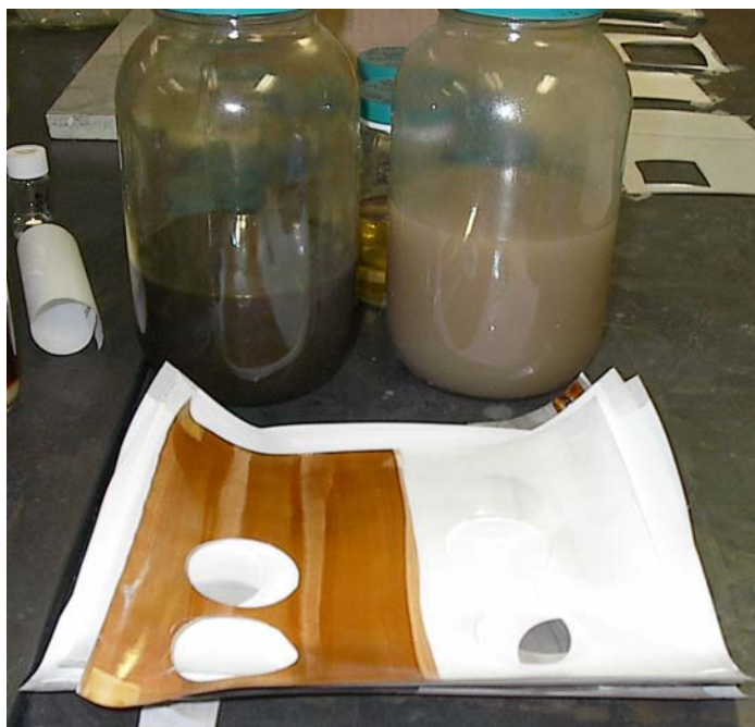
Figure 41. Comparison of Pebax ® 2533+80 wt% \text{AgBF}_4 coating solutions prepared with and without \text{H}_2\text{O}_2/\text{HBF}_4 stabilizer. Both solutions are >9 months old. The container on the right contains 0.5 wt% \text{H}_2\text{O}_2/\text{HBF}_4 . In the foreground are composite membranes as they appear immediately after coating PVDF support with the respective solution.
