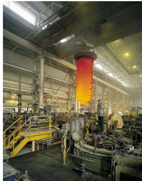
Figure 4: Sponge retort at TIMET, Henderson, Nevada. Source: TIMET.
