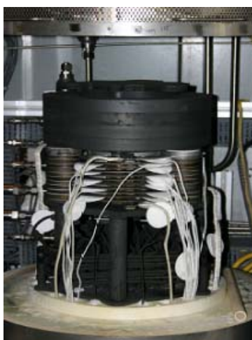
Figure 5-7 Image of the demonstration stack (U089, 10-cell) built in a testing furnace
