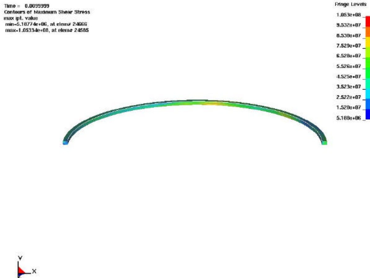
Figure 11. Shear Ring Maximum Stresses at 400 °F
