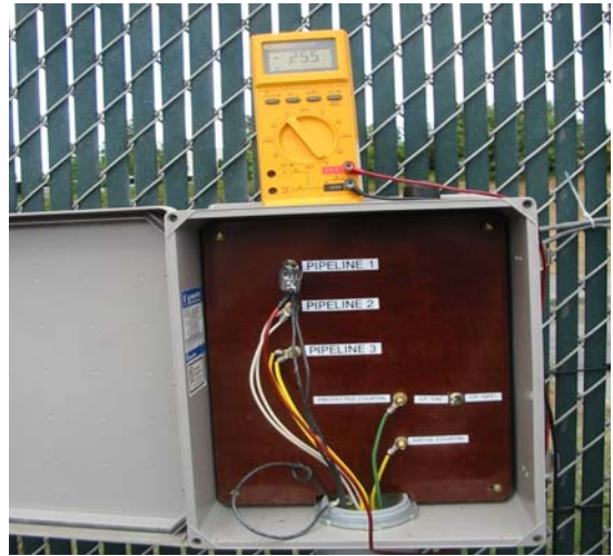
Figure 5- Junction box for measuring potentials of the pipe and coupons.
