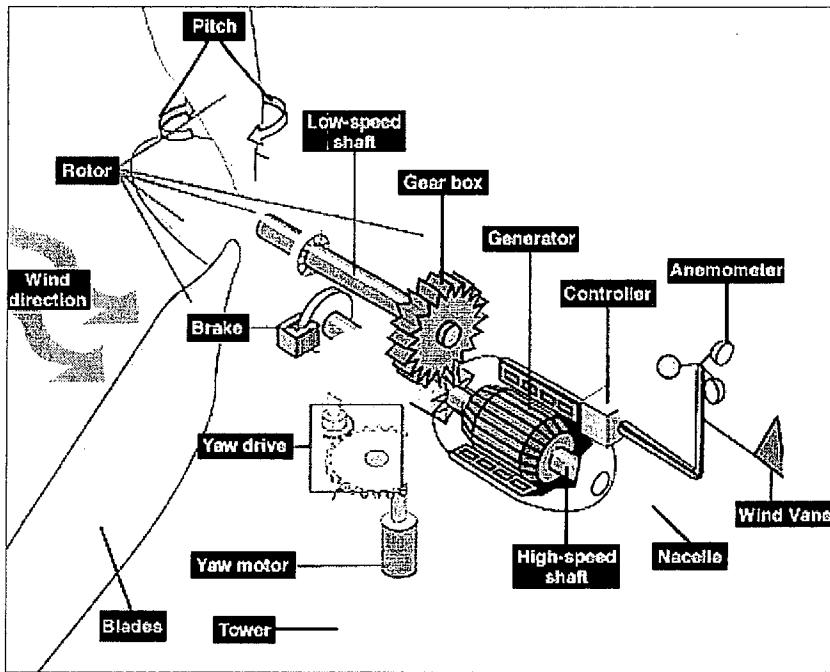
Figure 22: Diagram of a wind turbine. Wind turns the rotor, which may either be directly connected to the turbine or connected through a series of gears, as illustrated. The turbine generates the electricity, which may be stored in batteries when wind speed is insufficient to generate electricity.
