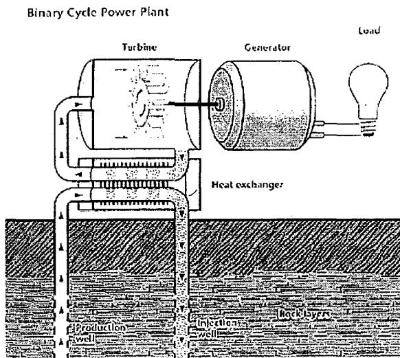
Figure 27: Illustration of a Binary Cycle Geothermal Plant. Fluids are injected through an injection well, heated by subsurface rocks, and recovered via the production well. The brine is then run through a heat exchanger where the hot brine converts Iso-butane to steam. The steam drives the turbine which drives the generator. Steam is then returned to the heat exchanger, where it is condensed and the process starts again. The brine is reinjected.
