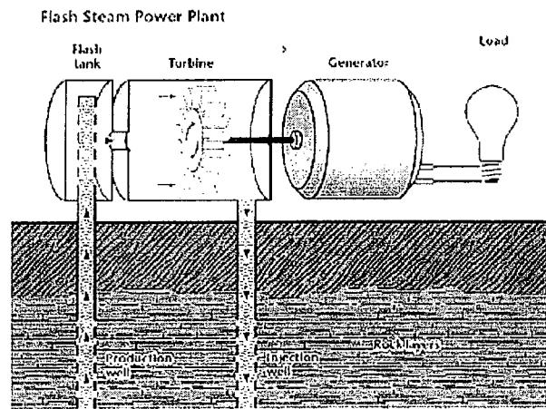
Figure 28: Diagram of a Flash Steam Power Plant. In this type of plant, brine is injected through the injection well, heated in the subsurface, and recovered through the production well. The brine is pumped into the flash tank, where the steam is drawn off to turn the turbine, which drives the generator. The remaining brine is reinjected.
