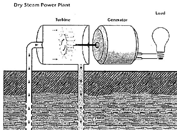
Figure 29: Diagram of a Dry Steam Power Plant. Brine is injected to hot rocks beneath the surface, where it is heated to steam. The steam is recovered through the production well and drives the turbine, which turns the generator.
