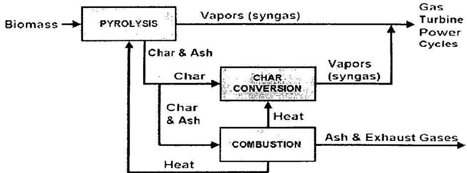
Figure 23: Diagram of a direct-fired gasification plant. (U.S. Department of Energy, [http://www.eren.doe.gov/biopower/bplib/library/li\\_gasification.htm](http://www.eren.doe.gov/biopower/bplib/library/li_gasification.htm))
