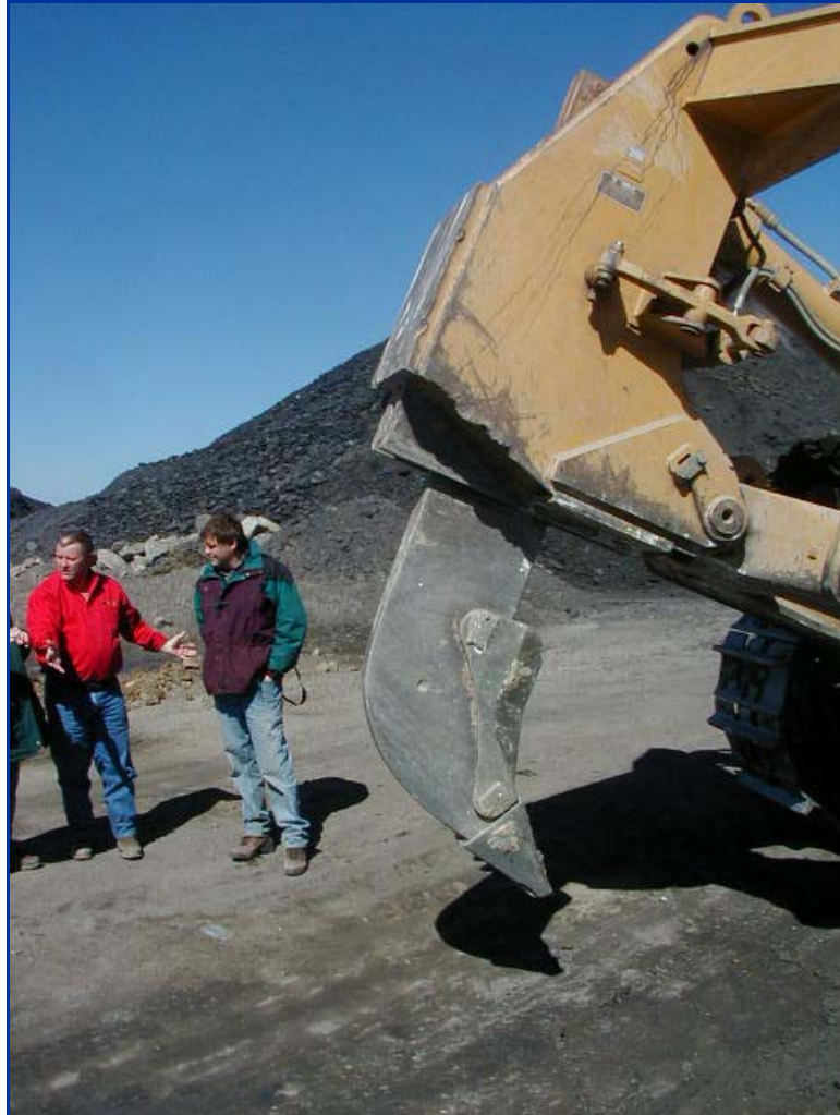
Figure 1.4. Example of a ripper attached to a D11 dozer.
