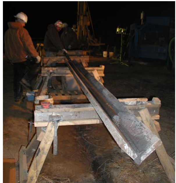
Figure 2. Photograph of lower Fort Yukon core removed from core barrel.
