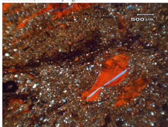
Figure 17E. Photomicrograph of grain mount from 1999.5 ft: Siltstone with oxidized organic debris. Quartz with lesser amounts of chert. White mica clasts. Matrix is silt, clay, and altered organic debris.
