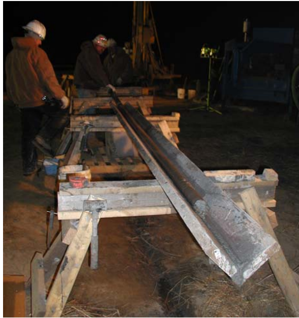
Figure 2.3 Photograph of lower Fort Yukon core removed from core barrel
