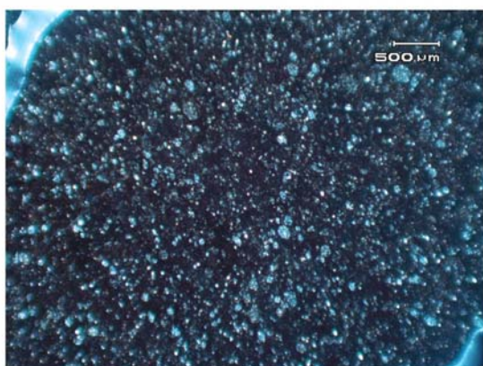
Figure 17C. Photomicrograph of cuttings from 2215-2225 ft: Conglomerate. Meta-siltstone clasts in grain mount. Grain mount clasts include sandstone, siltstone, chert with radiolarians, and cherty argillite.
