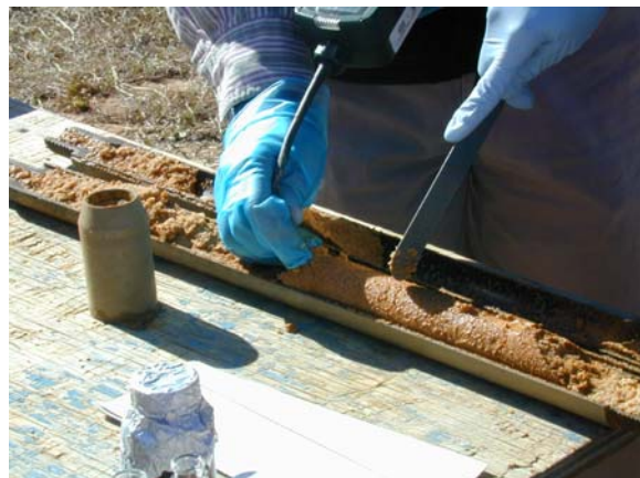
Figure 4.3: Photograph showing sampling of split spoon core.
